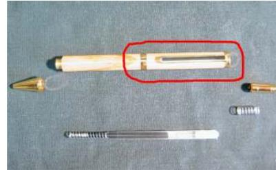
7. Insert the refill through the Pen Coupler and push the plastic mechanism towards the clip end until the threaded end of the back mechanism is close to the end of the plunger guide.
