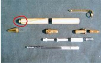
2. Press the Pen Centre Band, short end first, into the opposite end of the Lower Tube.
